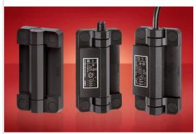
Similarly the CFSW-110 IP67 180° hinge which has been designed with its own built-in multiple safety switch, in order that in the event of accidental opening of a control cabinet door, machine panel or safety door, it automatically shuts off the power and protects the operators of machinery and production equipment. The CFSW is paired with its equivalent mechanical hinge, the CFMW-110 which facilitates a tough, safe installation.
